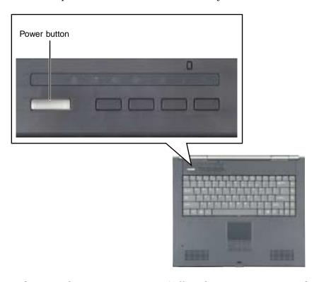
The power button is preset to On/Off mode. However, you can also set it to function in Standby/Resume mode. For instructions on changing the power button mode, see "Changing power settings" on page 158.
