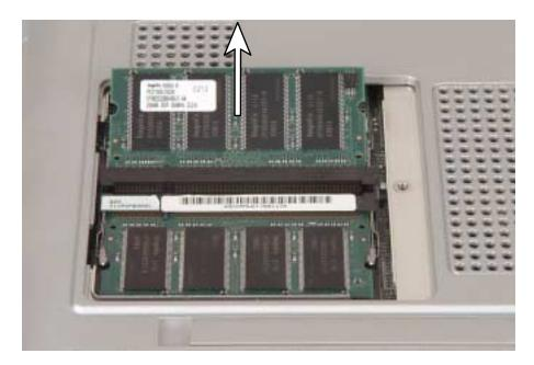
**9** Hold the new or replacement module at a 30-degree angle and press it into the empty memory slot. This module is keyed so that it can only be inserted in one direction. If the module does not fit, make sure that the notch in the module lines up with the tab in the memory bay.
