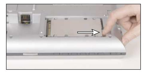
**8** Lift the end of the hard drive kit furthest from the connector, then remove the drive from the bay
